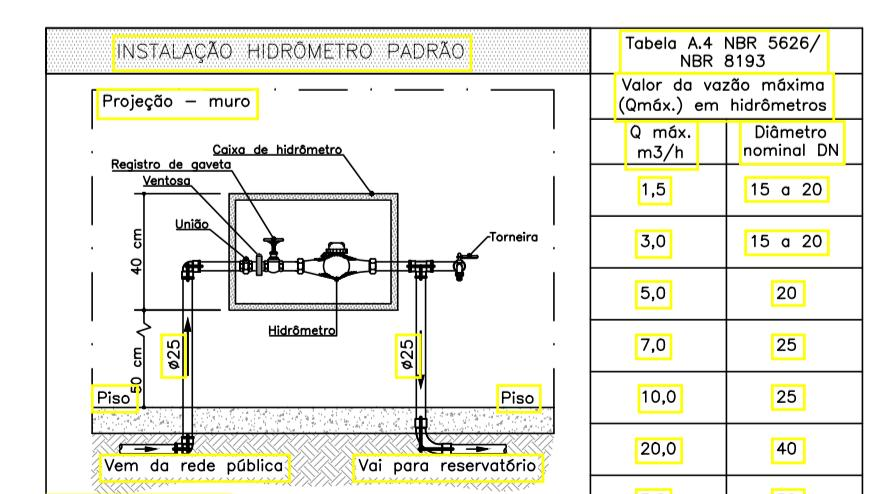
DETALHE 01 - CAVALETE HIDRÁULICO
